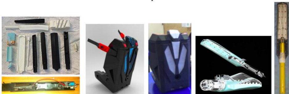
Figure 4. L to R: intermediate 3D printouts and electronic casings - toy bat only; Final renderings and images of completed product - both products
